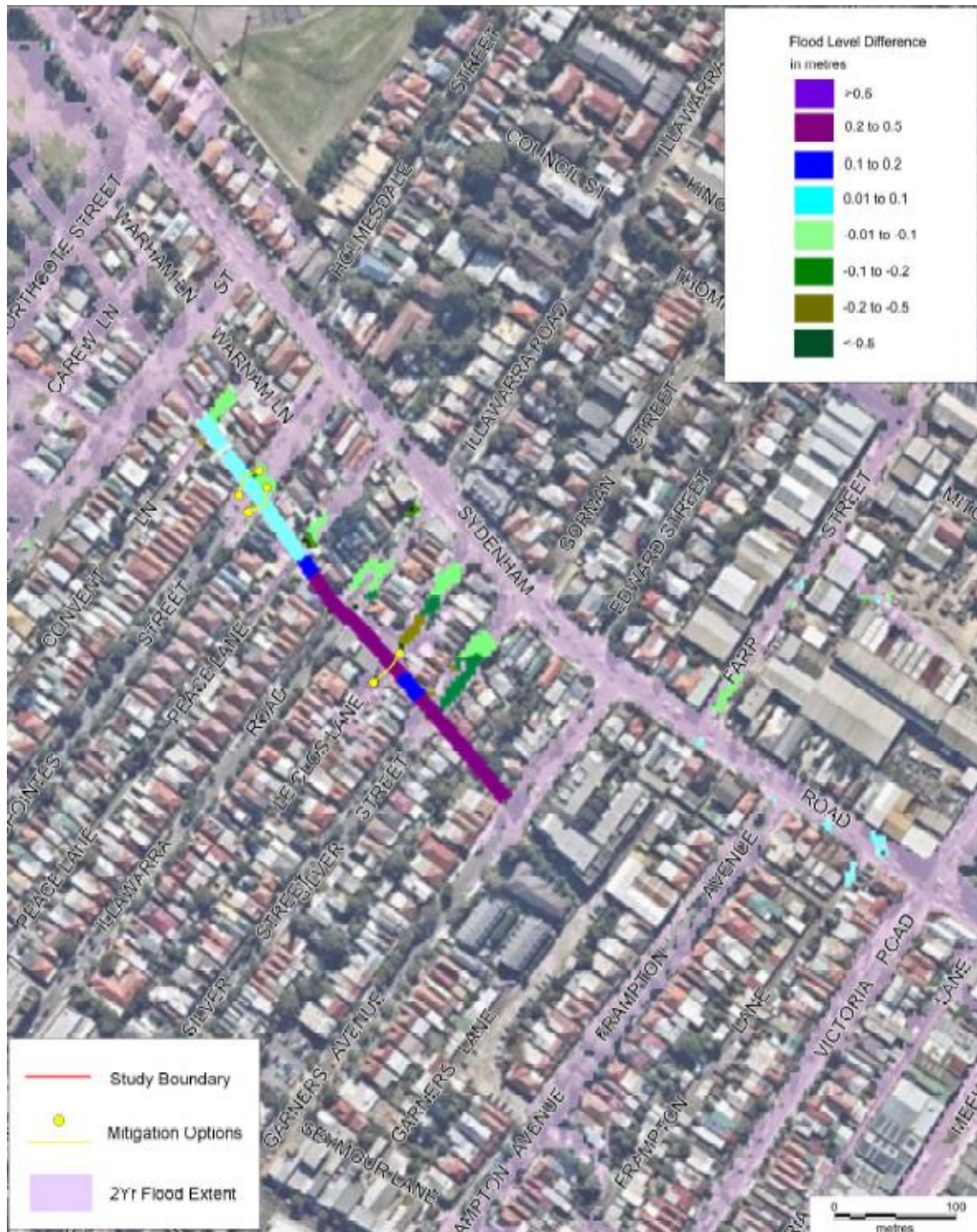
Figure 21 Works map – Inlet upgrade
